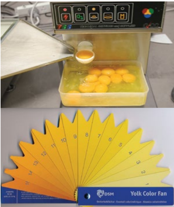
Figure 8 – Measurement of yolk colour using a yolk colorimeter or yolk colour fan
