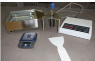
Portable equipment for measuring albumen height and Haugh unit
