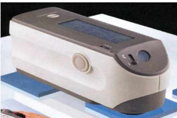
Konica Spectrophotometer used to measure the shell colour before and after staining
