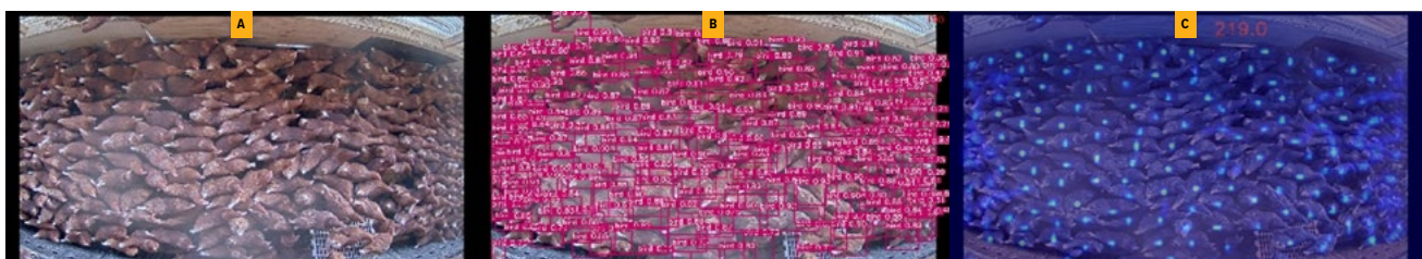
Figure 12: The visualisations of bird counting based on object detection and crowd counting. (A) The snapshot in a video frame; (B) The visualisation of all detected birds, annotated by the red bounding boxes; (C) The visualisation of dense counting, where each dot annotates a bird instance.
