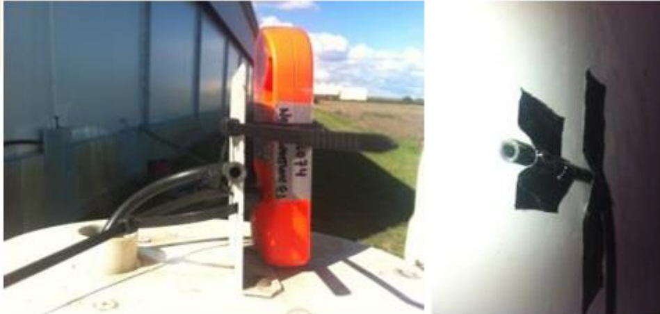
Photograph 17 - Rubber tube attached to the Stevenson screen (left) and inside shed (right)
