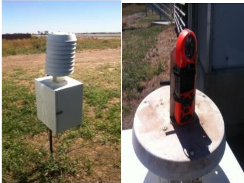
Photograph 16 - Stevenson Screen and Kestrel 4000 mounted outside shed
