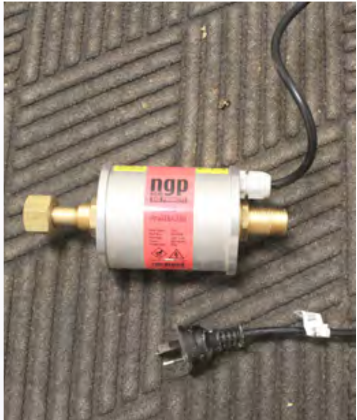
Photograph 10: CO 2 In-Line Heater Unit
