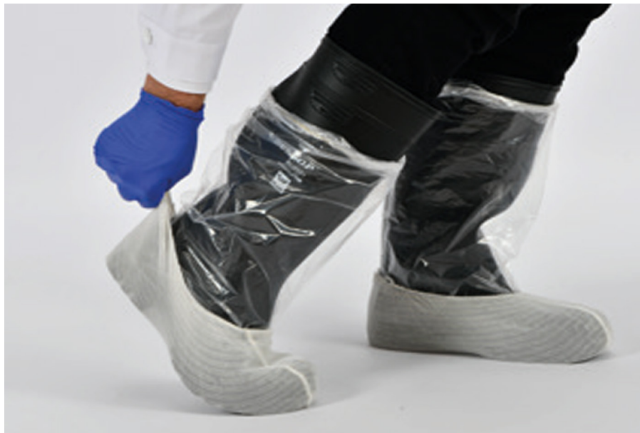
Figure 3. Put boot swabs over plastic boot cover (Romer Labs)
